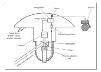
Fig-25 A typical Infra-scan Detector
