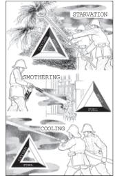
Fig-11 Triangle of Fire showing the three conventional methods of fire extinguishment-Starvation(A), Smothering(B), and Cooling(C)
