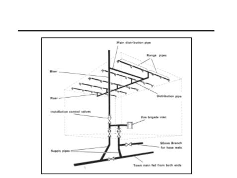
Fig-34 Diagramatic lay out of pipework of a sprinkler installation.
