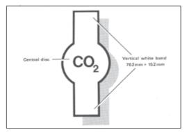
Fig-53 Standard warning symbol of a CO, Installation
