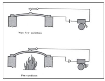
Fig-15 Heat detector using expansion of metal strip principle
