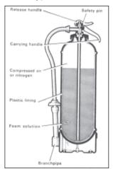
Fig-59-A Mechanical Foam Extinguisher (Stored Pressure Type)
