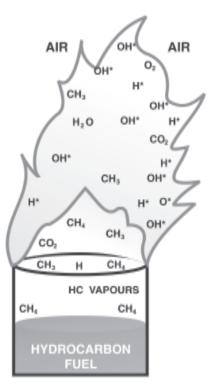
Fig-9 Uninhibited / Unbroken Chain Reaction showing active radicals like H<sup>\*</sup>, O<sup>\*</sup> & OH<sup>\*</sup> in the flame
