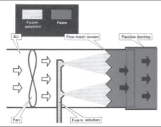
Fig-47 Principles of operation of a high expansion foam generator
