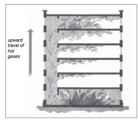
Fig-3 Showing how fire on a lower floor can spread to upper floors by convection
