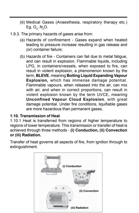
Fig-1 Showing methods of Heat Transmission (i) Conduction (ii) Convection (iii) Radiation
