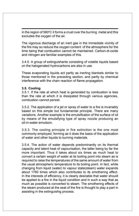
3.5.5. On the basis of thermal capacity and latent heat of vapourisation, water is an excellent fire extinguishing agent since both figures are high. For instance, the thermal capacity or specific heat of water is 4.2 kJ/kg/°C and latent heat of vapourisation is 2260 kJ/kg This fact, combined with its availability in large quantities, makes it by far the most useful fire extinguishing agent for general purposes.
